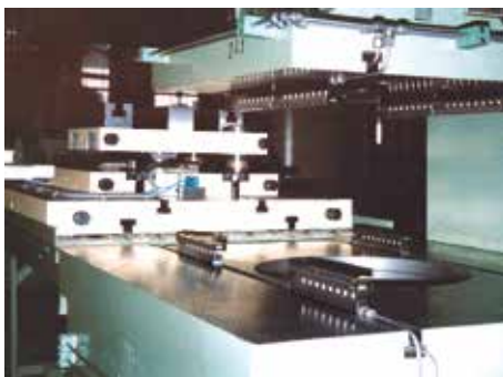
Double-T clamping bar on press bed and ram
