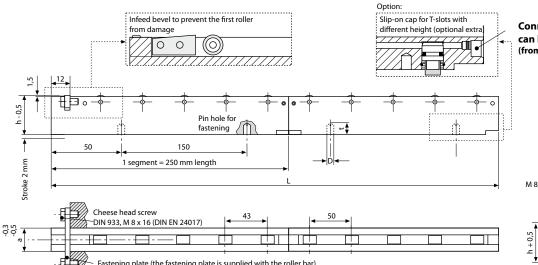
Connecting thread on both sides can be ordered as variant B (from L = 500 mm + preferred lengths)
