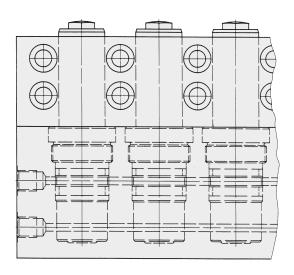
Double-acting threaded-body cylinders as pull-type cylinder for a multiple clamping fixture to mill a wrench flat
