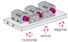
Clamping direction can optionally be in all directions vertically to the axis of the clamping lever. The clamping lever must be in retracted position and the cylinder cover must be rotated by the corresponding angle.
