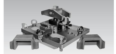
The clamping fixture in plate constructions installed on a vertical machining centre with rotary indexing table and trunnion bearing.
