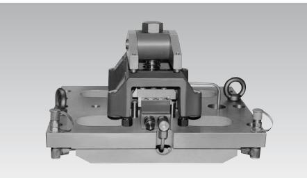
The opposite figure shows a hydraulicallyoperated fixture for concentric positioning and clamping of two casted housings, whose interior surfaces are due to functional reasons have to be concentrically arranged to the machined holes.
